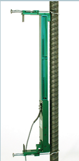
Model 3543 with 12 inch gauge length
