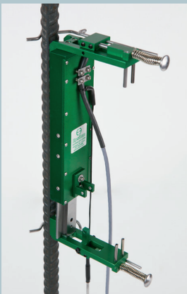
Model 3543 with 100 mm gauge length
