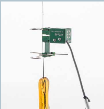
Model 3442 with 25 mm gauge length testing carbon fiber tow
