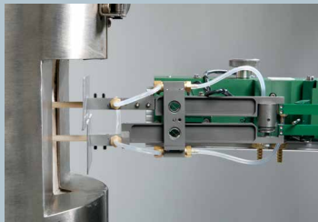
Model 3648 with 1 inch gauge length
