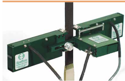
Model 3560-BIA with 25 mm gauge length
