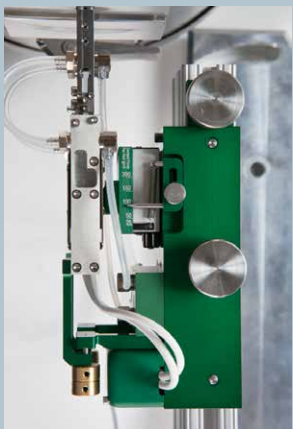
Model 3549 top view showing contact force scale for repeatable placement against test specimens
