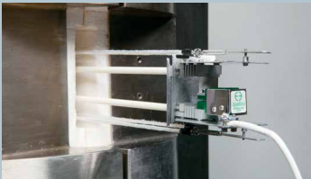
Self-supporting Model 3448 with clamshell-type materials testing furnace
