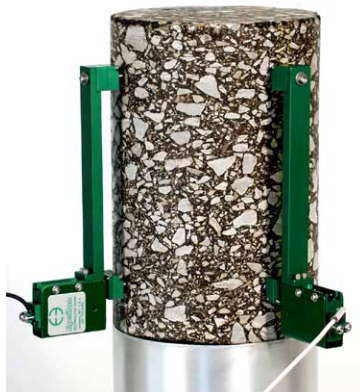
Model 3909-0400 with 4 inch gauge length
