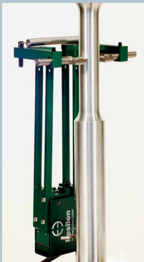
Model 3575 special long measuring range (custom model)
