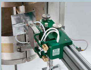
Model 3549 with 25 mm gauge length
