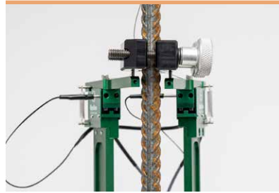
Model 3567 specimen attachment collar with extensometer installed
