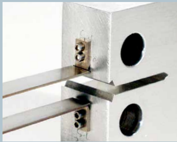
Model 3541 attached to bolt-on knife edges
