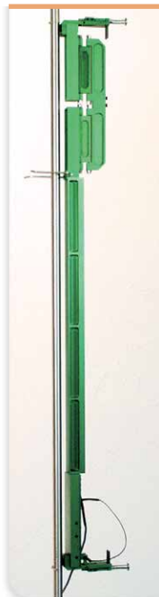
Special Model 3543 with ability to work on test samples that twist up to 15° during the test
