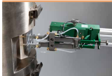
Model 3648 with 1 inch gauge length shown with a split furnace
